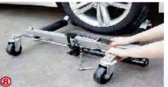
⑧ After finished the move for vehicle, Counter-clockwise to move the oil valve, pull out the safety pin, the car floor
