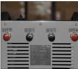
Independent 12V and 24V terminals ensure a safe and reliable connection
