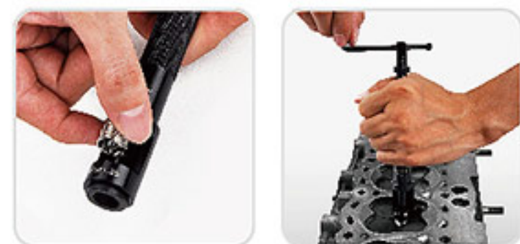
3. Load coiled insert into Coil Shielding Collar 4. Screw coil into thread slowly
