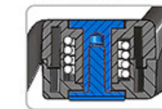
• Spring-loaded clamp holds funnel securely in position
