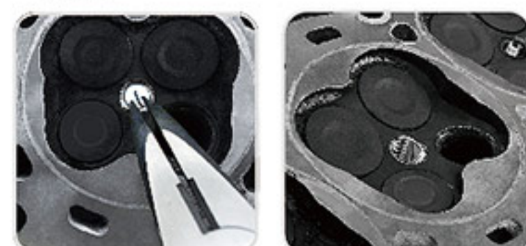
5. Use Pliers to take off pin on insert 6. Thread is repaired and ready to use
