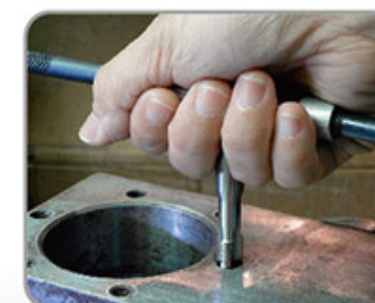
2. Tap re-drilled hole using tap
