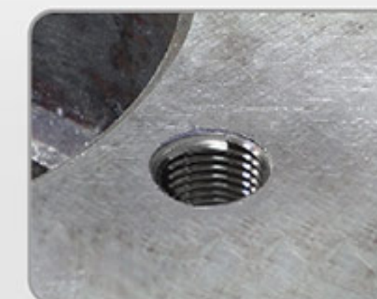
6. Thread is repaired and ready to use
