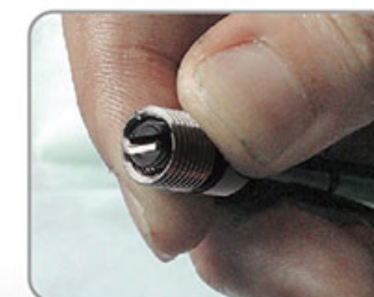
3. Load coiled insert into applicator
