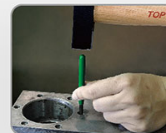
5. Using pin breaking tool, break off pin on insert
