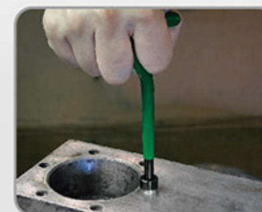
4. Screw coil into casting
